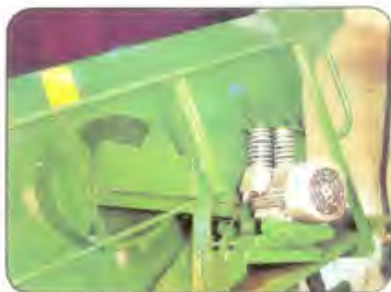
Electric drive. V-belt transmission.
