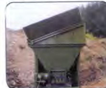
MD-feed hopper with belt feeder Hopper capacity 6 cbm. Belt feeder 2.2 m x 650 mm with 5.5 hp standard motor.
