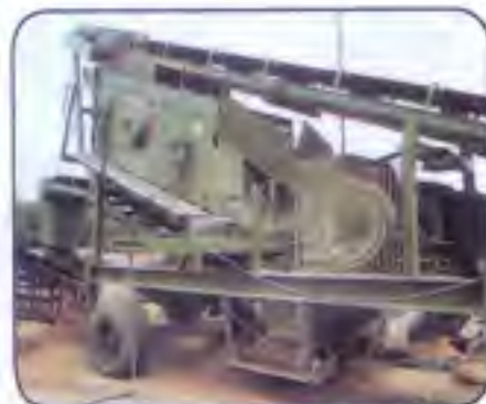
Tarek A 1230 with jaw crusher: - max. crusher weight 6 tons - bypass to main conveyor.
