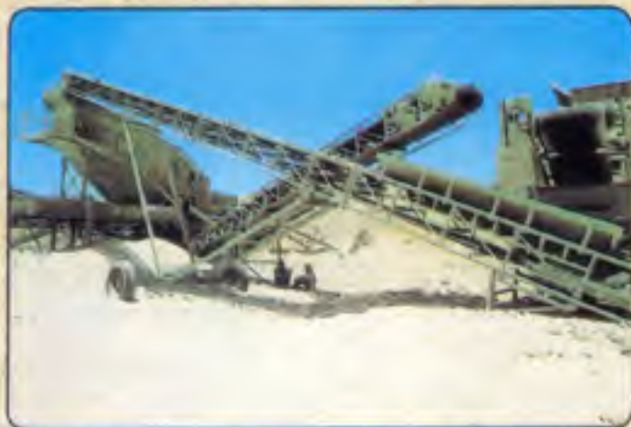
19 m x 800 mm. Capacity 325 tons per hour mounted to a mobile adjusted chassis type M2. Entering into the crusher for transportation between primary and secondary plant.
